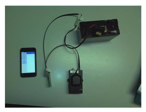
If your FLARM unit is already powered with a RJ cable, and you do not want to change the wiring, move the power cable from your FALRM unit to the Disp port of the SoarTronic BT1 module. Then add another IGC RJ cable to connect Flarm port of the SoarTronic BT module to the MiniBox or original FLARM
