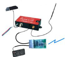
You can add the SoarTronic Bluetooth module between RedBox and the external display. You will need another RJ12 cable, that is identical with the cable originally between the RedBox and ExternalDisplay.
