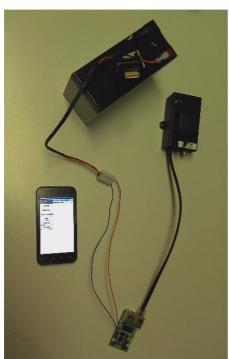
If you use MiniBox or original FLARM units, you have to feed operating power to your device using the same RJ connector as you use for data communication. To make installation easier, you can connect the 12V operating power to the SoarTronic Bt module. BT mnodule then connects the Vin and GND into IGC standard pins of the RJ connector. (this 12V is NOT used to power the BT module). Olease note, that the BT module does not have build in reverce current protection or fuse.
